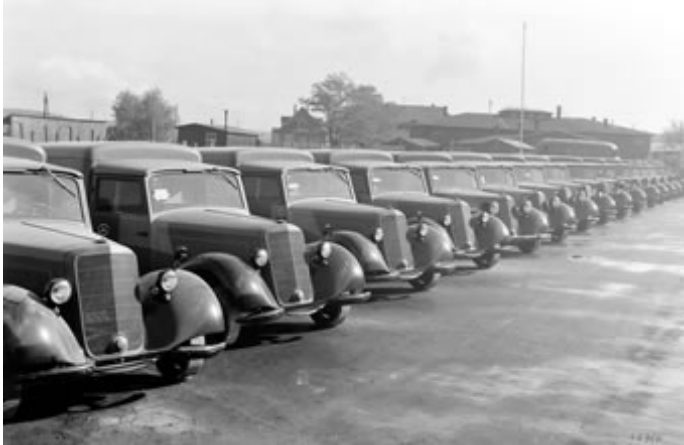
Mercedes-Benz 170 V panel van, 1946 (the first four vehicles from the left feature the small headlights of the first generation)
